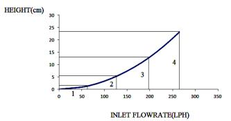
Figure 4: Piecewise Linearization of Input and Output Characteristics
