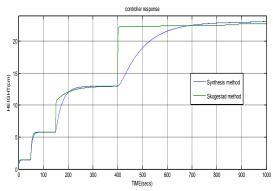
Figure 5: Comparison of Direct Synthesis and Skogestad Methods
