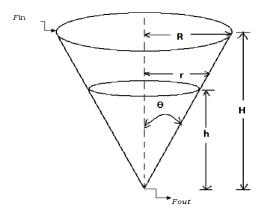
Figure 1 Structure of Conical Tank
